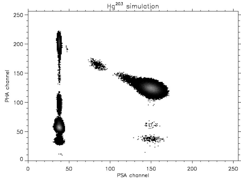
Effectiveness of the Pulse Shape Analysis (PSA) for the phoswich detectors of the BeppoSAX/PDS instrument
