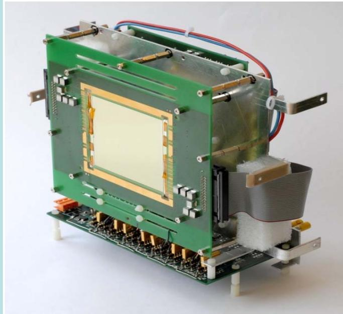
The 8 single-anode channels laboratory prototype with discrete front-end electronics (the flight version will be MUCH more compact!)
