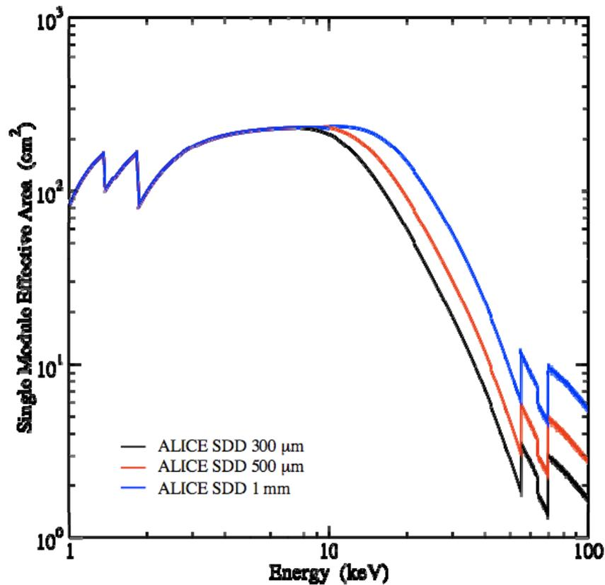
Efficiency  $\sim 1$  up to 10 keV, can be increased in the range 20-100 keV with thicker detectors
