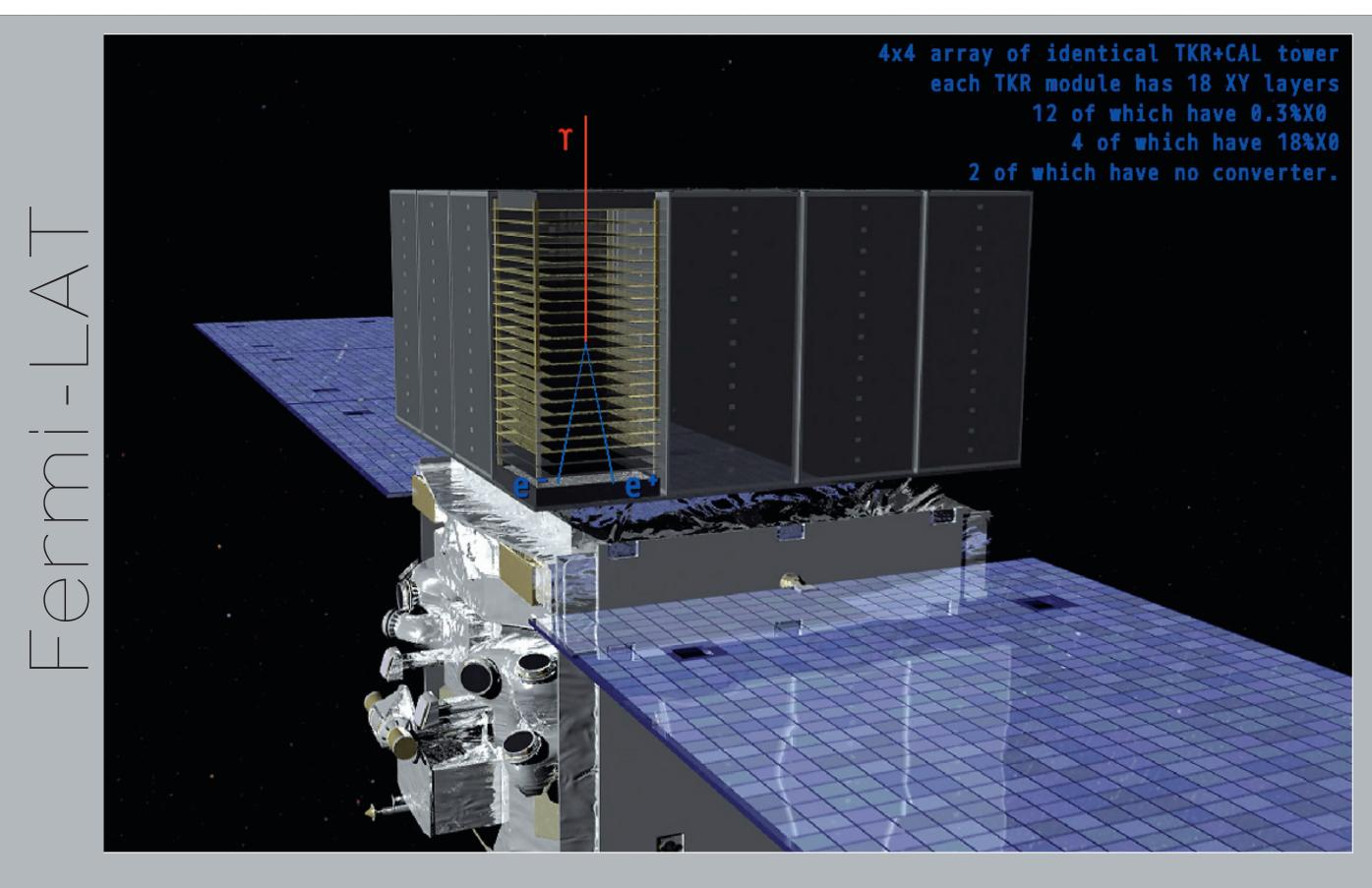
The Fermi Gamma-Ray Telescope, launched on June 11th 2008 from Cape Cañaveral, performs gamma-ray measurements over the whole celestial sphere. The LAT measures the tracks of the electron and positron that result when an incident gamma ray undergoes pair conversion in a thin, tungsten foil, and measures the energy of the subsequent electromagnetic shower that develops in the telescope's calorimeter. Energy range: 20 MeV to > 300 GeV. Angular resolution ~ 0.1 deg above 10 GeV.
